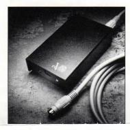
The infrared receiver connects by cable to the keyboard jack or serial port of the computer. It uses a special data verification technique to understand transmissions from the TOTEBOARD. Those transmissions are then relayed to the computer. Connecting the Receiver to the serial port allows use of both the standard keyboard and the TOTEBOARD. It can be used up to 30 feet away from the Receiver, which has selectable switches for use with IBM PS/2, AT, XT, PC and compatible computers.
