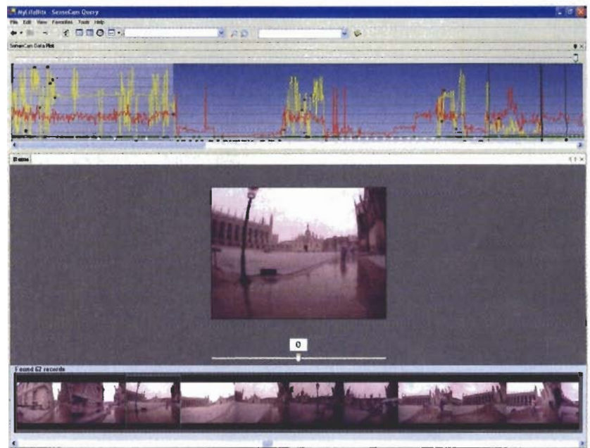
AWAY-FROM-HOME MOVIES: A SenseCam will take a photo every minute or whenever its sensors detect a change in the environment, such as lighting or temperature. A chronological sequence drawn from the 1000 to 2000 photos taken in an average SenseCam day is at the bottom. At the top is a plot of the data points captured by the various sensors.
