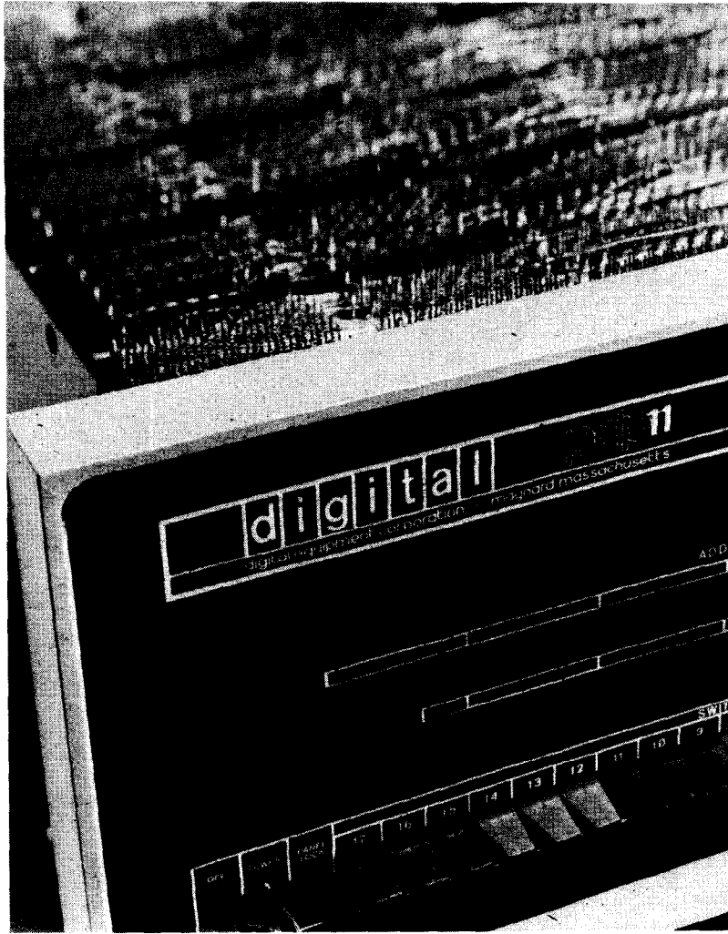
The PDP-11 has adopted a modular packaging approach to allow custom configuring of systems, easy expansion and easy servicing.
