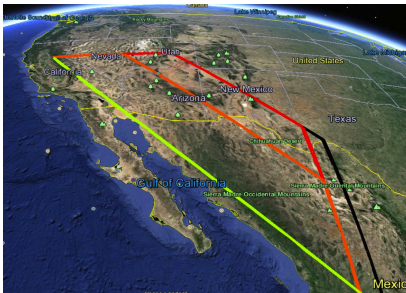
Figure 7: The path in black is the oracle plan from start (lower right corner) to goal (upper left corner), red is the Replan by Sampling plan which comes close to the oracle plan, orange is the Replan by Mean plan which in this case is worse than Replan by Sampling by 236 seconds. The green path is the plan taken by Linear Interpolation and No Replan which are both happen to be going straight for the goal in this example.
