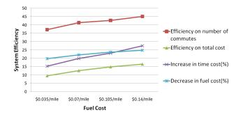
Figure 3: Effect of fuel cost on the efficiency of ABC system. Increasing fuel costs improves the efficiency of ridesharing.
