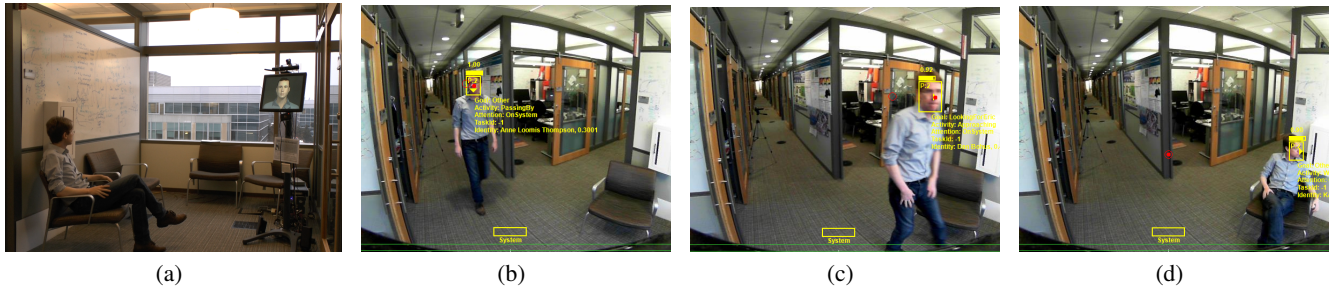
Figure 2: (a) The Assistant outside the owners office. (b) Visitor walks through the Assistant’s field of vision. (c) Visitor heads towards the chair to wait for owner. (d) Visitor sits down in Assistant’s field of view.
