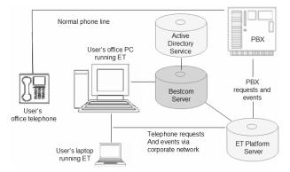
Figure 5: A high-level overview of the implementation architecture for the ET, showing the overlaid Bestcom service. The field deployment consisted of four PBXs and four Windows servers.
