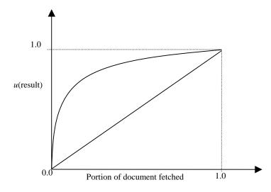
Figure 1. Linear and nonlinear utility models for representing the value of prefetching portions of documents into the local cache as a function of completeness of a download. The nonlinear curve captures the notion of decreasing marginal returns with additional fetched content.
