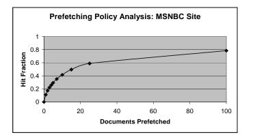
Figure 4. Analysis of the value of prefetching using a Markov model built from a training set of log data. The graph displays the probability of content from the next document accessed being in the cache as a function of the number of documents prefetched.
