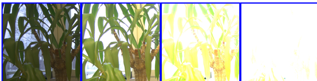
Aggressive tree compression in \log(\text{RGB}) space (input/output/diff/tree) and remaining residuals encoded in a low dynamic range DXT-compressed texture:
