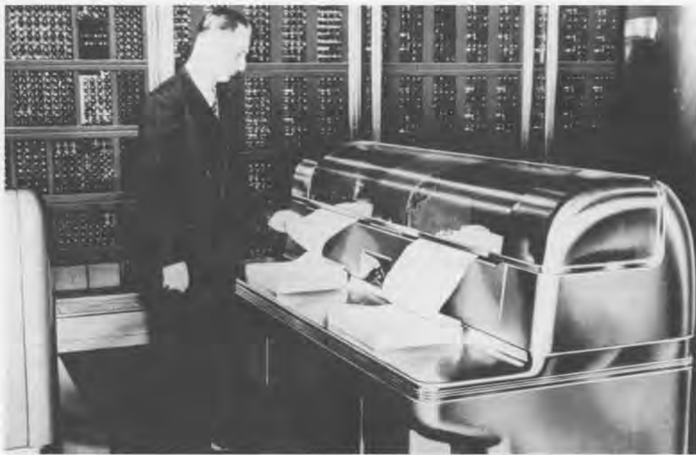
The SSEC used conventional IBM 405 tabulators rehoused with the tape slugs turned upside down, and the wires crossed so as to make it work out of the back instead of the front for the sake of appearance. The 12,000 inch and a quarter diameter 25L6 boggles out of which the arithmetic circuits were made can be seen in the back of the photo.
