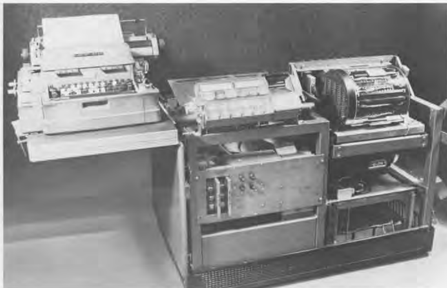
The LGP-30 was one of the many small scale drum computers sold in the fifties. Built in 1956, in 1962 it rented for $1300 a month. The drum on the far right held 4K bits of information.
