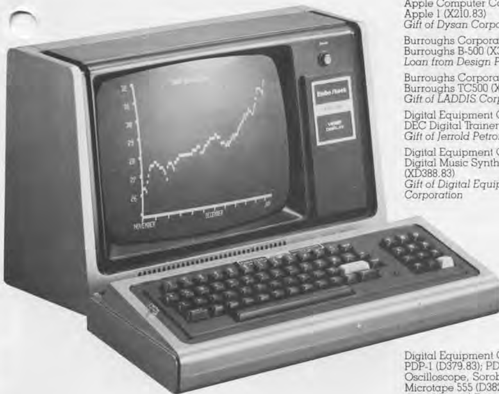
TRS-80. TRS-80 Model I's, like the one pictured here, were introduced by Tandy Radio Shack Corporation in 1977. During that same year the Apple II and the Commodore Pet 2001 were introduced, establishing the first three personal computer designs to come assembled with BASIC built into the firmware, which allowed them to achieve a BASIC operating mode on power up. The TRS-80 Model I is one of several PC's that will be featured in the Personal Computer exhibit when the Museum opens November 14, 1984.
