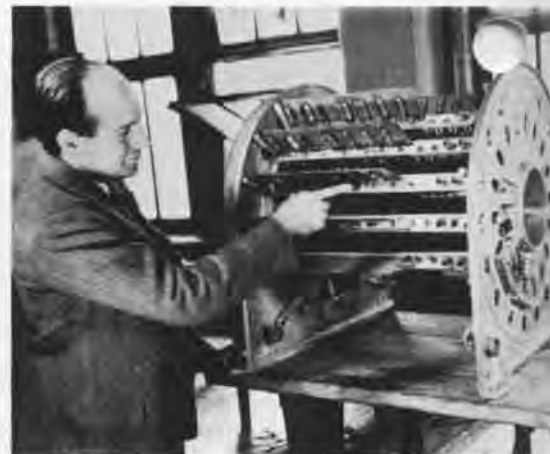
J. Presper Eckert Jr. is shown with a BINAC Mercury Memory Tank.
