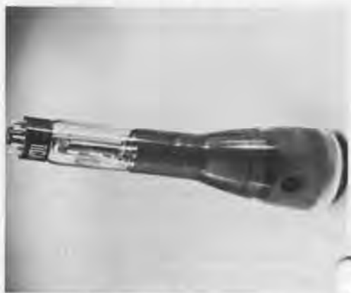
Figure 1. An early RCA cathode ray tube that could have been used for storage.
