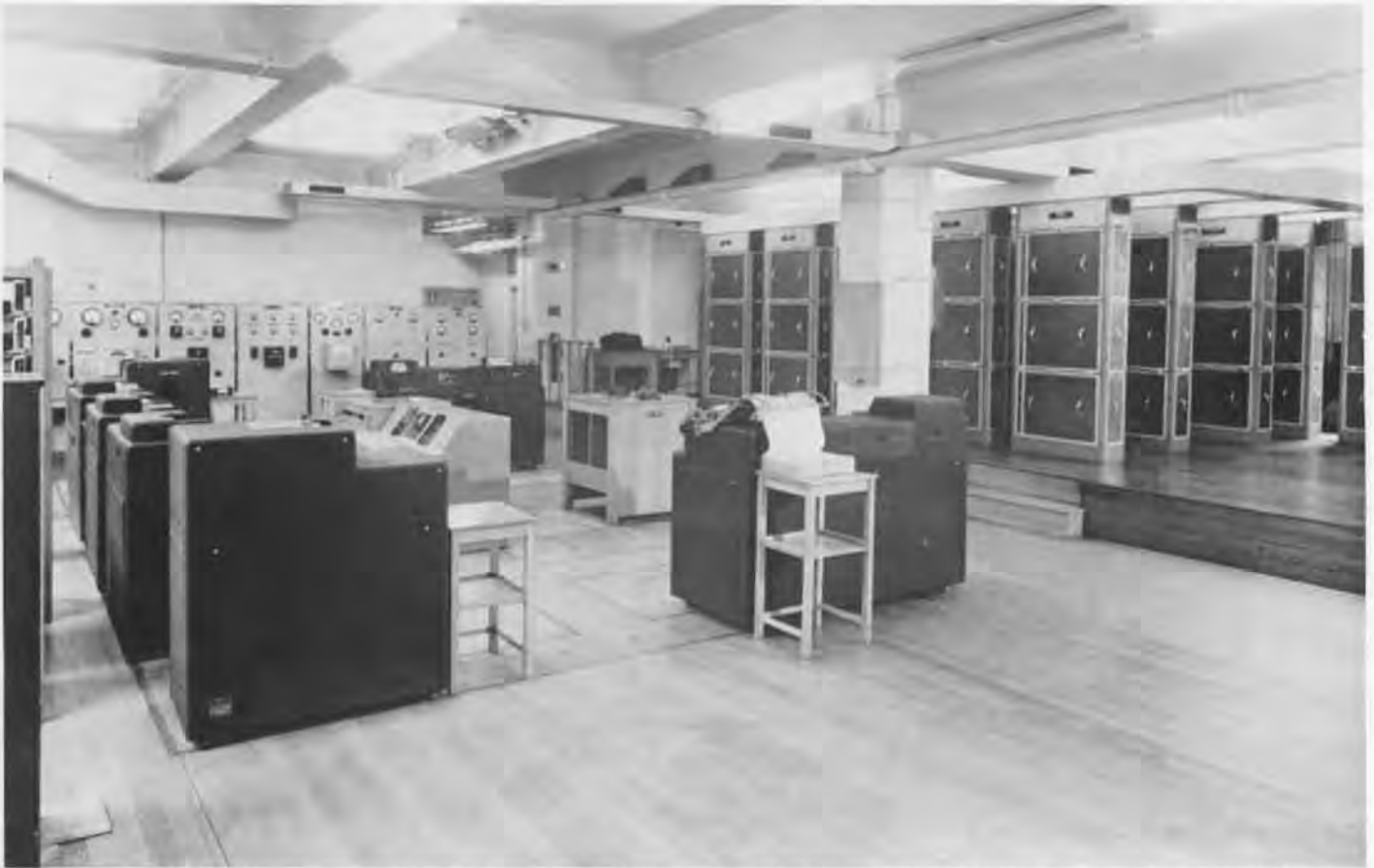
The LEO I used 5,000 valves (vacuum tubes), drew 30 kw of power of which 3 kw were used for cooling fans, and occupied a room 45 feet square. The mercury in the delay tubes weighed half a ton. It executed 700 instructions per second and could produce two-line papyrus at the rate of 50 per minute on the line printer.
