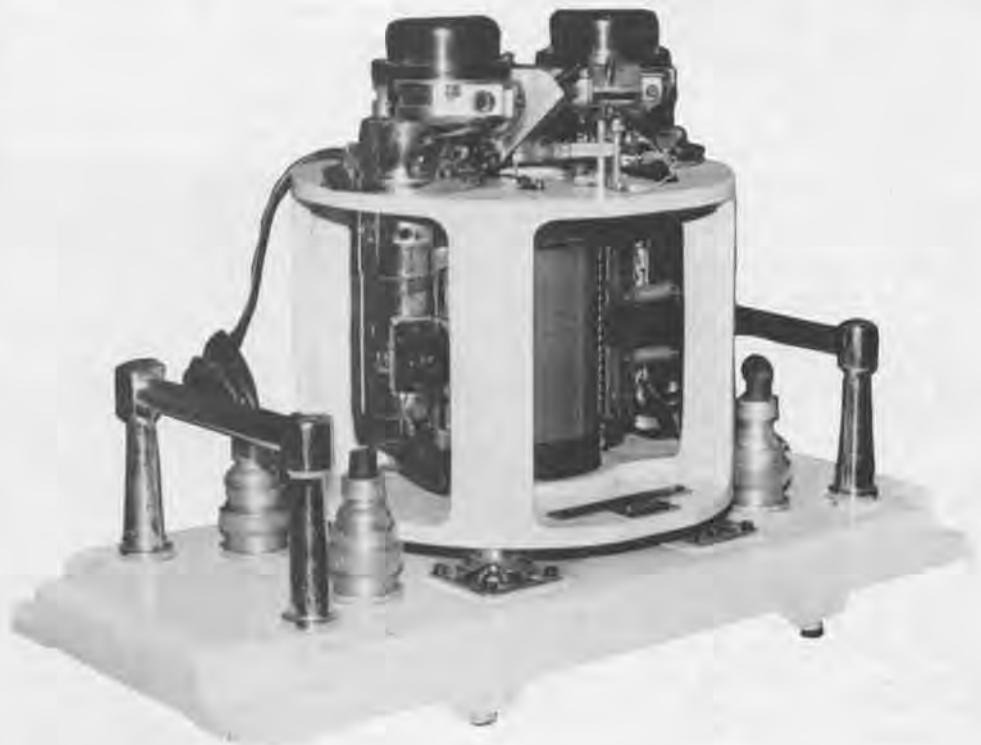
Drum from the English Electric Deuce. Built in 1957, the Deuce drum stored 8K \times 32 -bit words on 256 tracks of 32 words each. It measured four inches by six inches; most first-
