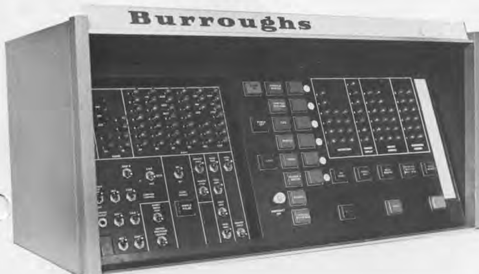
Burroughs B-500. The front control panel of a Burroughs B-500 Central Processing Unit. Released in 1968, it was the small-scale end of the Burroughs "500" family.
