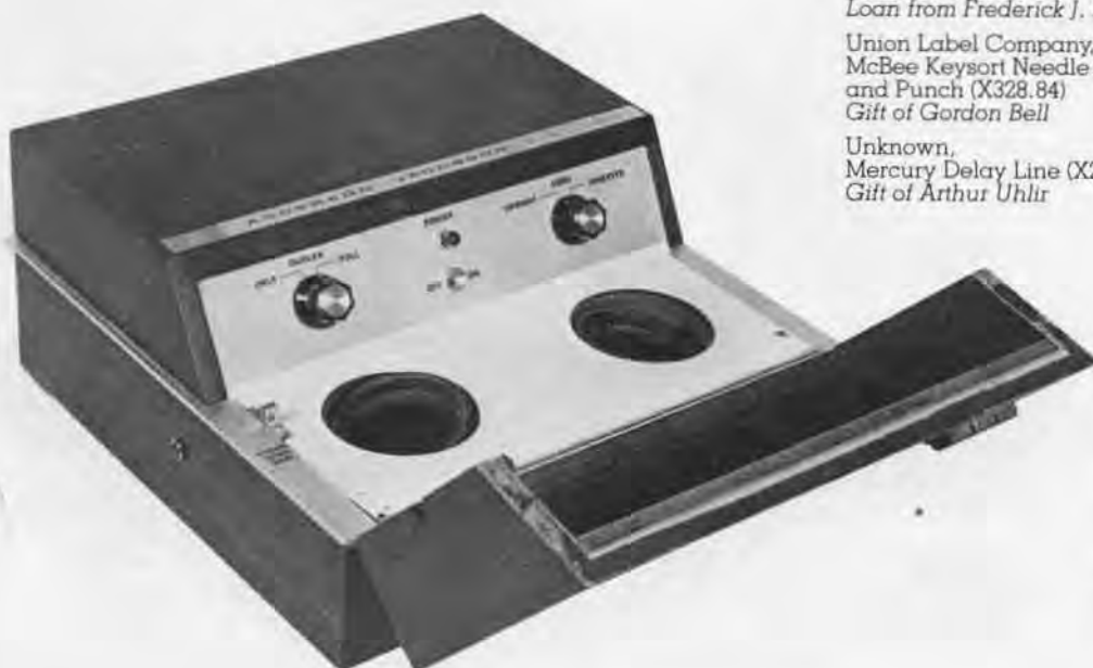
Acoustic Data Coupler. This Anderson Jacobson Acoustic Data Coupler 260 (circa 1963) is one of the earliest modems. A modem is an acronym for MODulator DEModulator unit, a device that converts data from a form that is compatible with data processing equipment to a form that is compatible with transmission facilities, and vice-versa.
