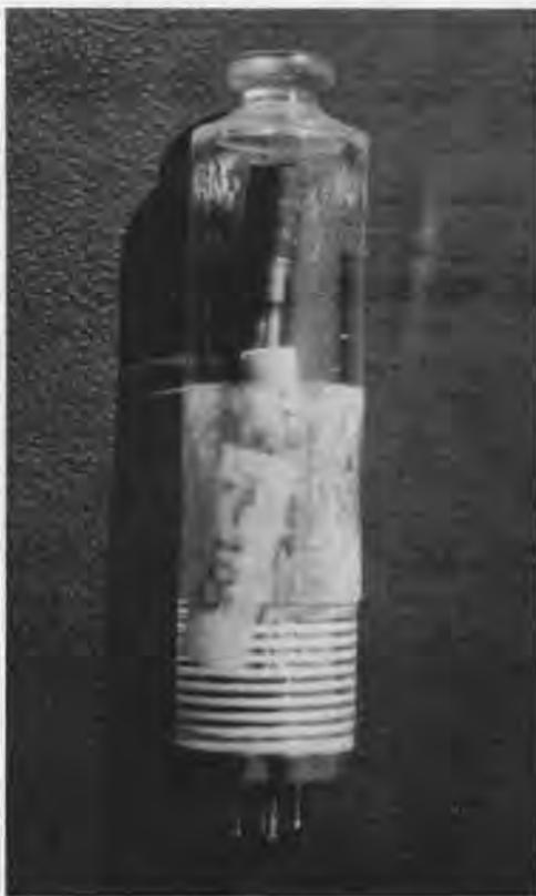
TX-0 transistor. The first TX-0 transistors were in tubes to make it easier to test and replace them. The TX-0 had only 12 transistor failures, and almost every transistor that lasted more than 500 hours is still operational today.
