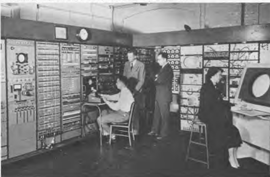
The Whirlwind console room in 1951 with the marginal checking and toggle-switch test control panels on the left. Stephen Dodd, sitting at an input device, is being watched by Jay Forrester and Bob Everett. Ramona Ferenz is seated at the prototype display to monitor the Cape Cod system, the prototype for SAGE.
