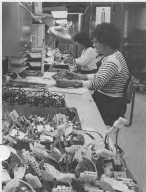
A large part of computer manufacturing is not robotized, but people assemble, wire and test the components that make up a machine. This photo is from a Data General prototype assembly plant in Westborough, Massachusetts.
