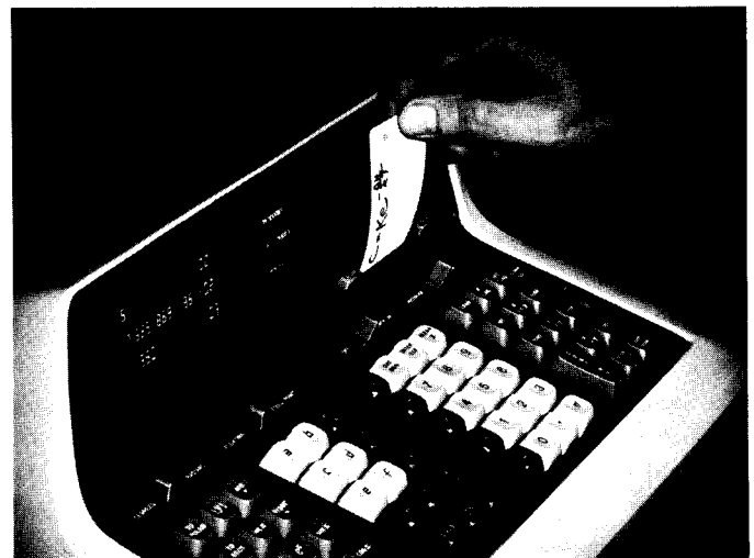
Fig. 8. Programs can be entered into the calculator by means of the magnetic program card. The card is inserted into the slot and the ENTER button pressed.
