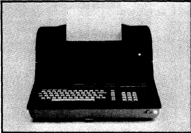
Fig. 7. Model 9866A Thermal Line Printer is the primary output peripheral for Model 30.
