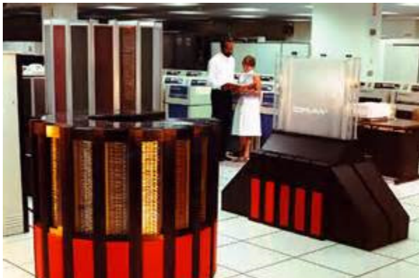
Figure 9 Cray 2 with Fluorinert cooling
