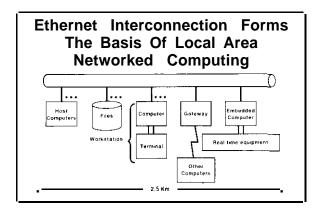
Ethernet is an extended bus. Up until now busses have provided high-speed computer communications within a very limited area-a single cabinet or room. Ethernet provides an extended bus that will link information processing nodes throughout a building, campu or industrial complex
