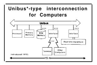
If you look at current computer architecture you will find standards. One such standard is the Digital Unibus that defines the architecture used in the large selling series of minicomputers ever built-the PDP-11 series. The Unibus standard made it possible for our users and a number of different manufacturers to built memory boards, communications interfaces, and other components that can be plugged directly in a PDP-11 system in an open-ended fashion.
