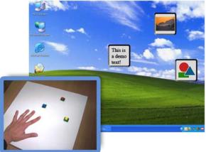
Figure 3: The clipboard content can be viewed by pressing on the surface, with thumbnails shown in a layout corresponding with the spatial layout of the physical interface.
