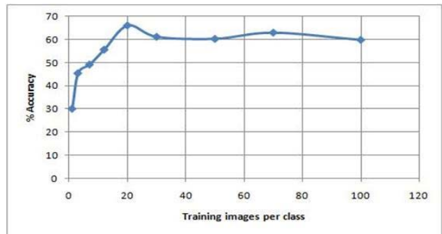
Figure 8. The testing accuracy of fully supervised trained ensemble classifier with different number of training examples.
