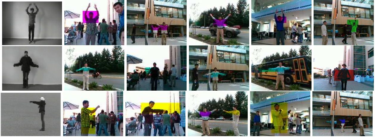
Figure 3: Examples of detection results. Each row shows an action class: hand waving (first row), hand clapping (second row) and boxing (third row). Each image is a sample frame from the action video. The first column shows the training videos from the KTH dataset. The second to the fifth columns are some detection results. The highlighted bounding boxes correspond to the detected spatial window W^* and we apply different colors to distinguish different action types: clapping (turquoise), waving (magenta), and boxing (yellow). The final column gives the miss detection examples, where the bounding boxes are ground truth labeling: clapping (red), waving (green), and boxing (blue).
