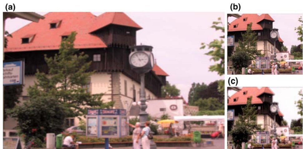
Fig. 1 a Shows a blurry picture with a resolution of 2,592 \times 1,944 reproduced in 3R photo size. b Is the naïve preview image in a resolution of 400 \times 300 on a 2 in. display. It looks without image blur. c Shows our perceptual preview image after structure enhancement and blur visualization
