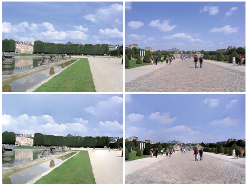
Fig. 4 Examples of structure enhancement. The first row shows two naïvely reduced images, with many details of trivial interest. The second row shows the structure enhanced images. Our method flattens subtle edge regions, while boosts strong edges
