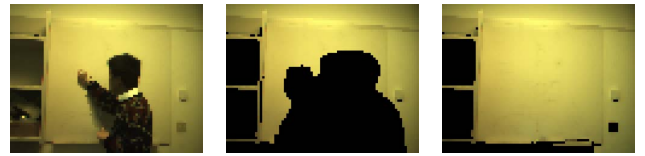
Figure 4: 1) Colors of the cell images. Note that the strokes on the whiteboard are removed by our background color estimation algorithm. 2) Colors of the cell images that go into the Update Module. Note the black regions contain the cell colors that are filtered out by both the change detector and the color estimator. 3) Integrated whiteboard color model.
