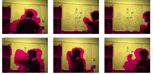
Figure 5: Samples of the classification results. The images above correspond to the images in Figure 2. The classified foreground region is tinted in purple and is larger than the actual foreground object due to motion, shadow, and spatial filtering.
