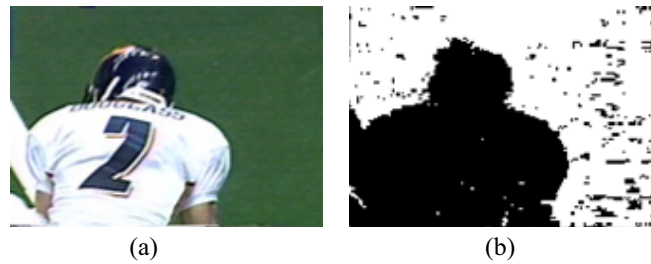
Fig. 5. Samples of close-up detection. (a) A close-up frame. (b) Masked image to detect whether there are heavy black blobs
