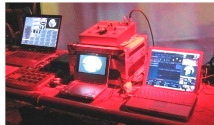
Figure 1: Typical VJ set up, showing laptops (running Resolume and Modul8 software), video mixer, monitor and other peripheral devices.
