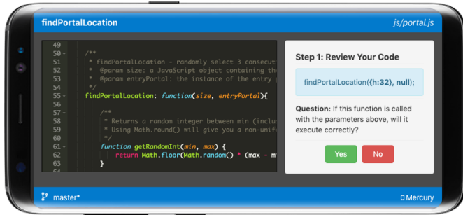
(c) Step 1 of Grounded Microtasks ask the user to assess the behavior of a function with a particular set of function parameters.
