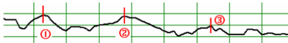
Figure 2. Sub-shot boundary detection by finding local maximum of frame difference curve (three boundaries are found for this shot).
