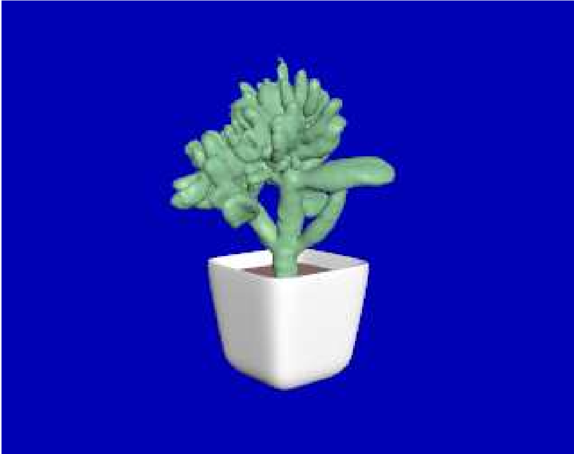
Figure 14: Modeling a Jade Plant from MRI data – The jade plant surface was modeled by extracting an isosurface through interpolated MRI data, using GENMOD’s implicit surface approximation capability.
