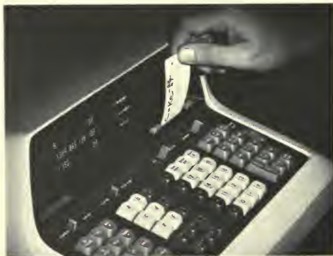
Fig. 8. Programs can be entered into the calculator by means of the magnetic program card. The card is inserted into the slot and the ENTER button pressed.
