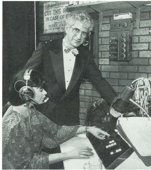
Gordon Pearlman, who designed Broadway's first computerized lighting control board, visits his LS-8 "Sam," reconstructed as it was in the Shubert Theater in the 1970s. Hooked up to a Digital PDP-8, Sam lit A Chorus Line for nearly 13 years.
