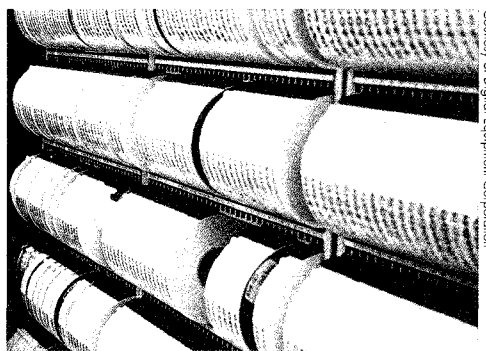
This is a computer's “library.” The reels of tape magnetically stored volumes of information in a form the computer could read.
