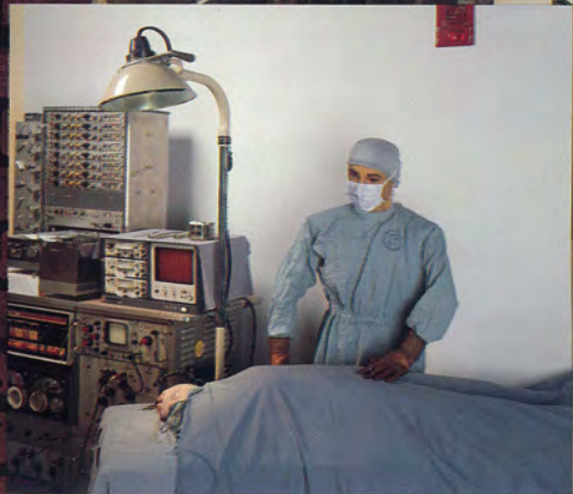
The rack of equipment to the left of the operating table contains a PDP-8e minicomputer.
