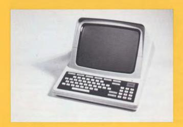
La Radiotechnique terminal, one of many used with France's successful telecommunications network.
