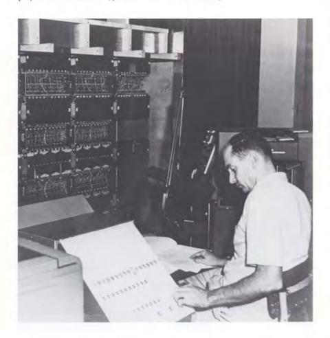
Testing of the Johnniac involved programming the computer to work on an endless calculation while workers checked each connection. A memo from this time states, "Applications for wire-wrigglers now being accepted."
