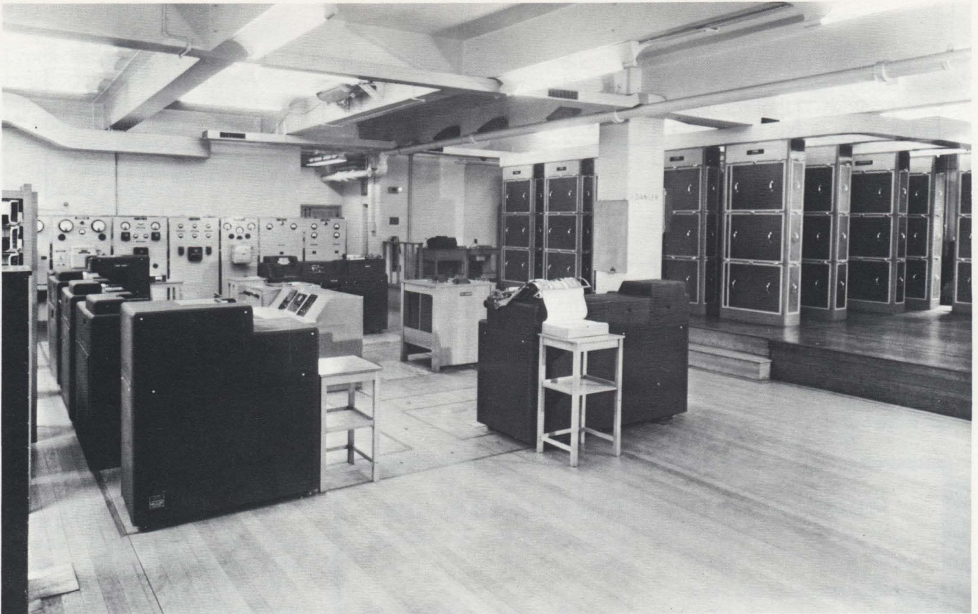
The LEO I used 5,000 valves (vacuum tubes), drew 30 kw of power of which 3 km were used for cooling fans, and occupied a room 45 feet square. The mercury in the delay tubes weighed half a ton. It executed 700 instructions per second and could produce two-line payslips at the rate of 50 per minute on the line printer.
