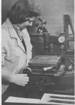
Dimensional Check. The machine die and the weight of the pressed cores had to be continually monitored to insure maximum uniformity of core size. Before each press run a dimensional check was made with a toolmaker's microscope in order to assure quality control.
