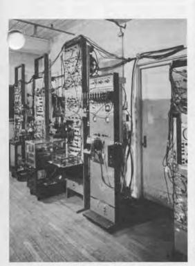
Pulse Testing. A sample of 50 cores from each lot was used for hysteresis-loop measurements. The test equipment for pulse testing and miautomatic selection testing consisted of an electronic core counter, an evaluation pulse tester, fully automatic and semiautomatic core testers, and a plane tester.
