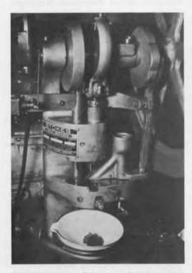
Core Pressing. After five days of getting the material ready for making cores, core pressing was done automatically by a Stokes press which was capable of 60 pressing operations per minute.
