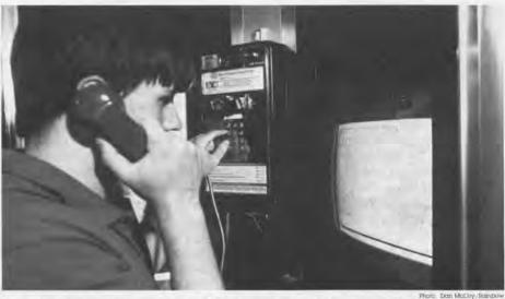
The computer direction assistant holds a road map of 11 square miles of Boston and Cambridge and can find the quickest route between any two points on its map. Visitors communicate directly with the computer via a touch-tone telephone. The assistant is very forgiving of mistakes and provides instructions in good, clearly-spoken English.
