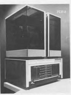
In April 1965, the idea of the minicomputer was realized with the delivery of the first PDP-8. The processor of this Classic Eight was housed in a transparent box revealing the elegance of its logic modules.
