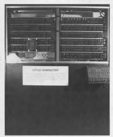
0000000001 Little Character, by Control Data Corporation, 1959. The Little Character was a prototype computer developed to test the concept of modular circuit design at Control Data Corporation shortly after its incorporation in August 1957.
