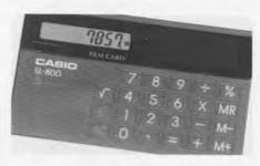
The SL-800 Film-Card announced by Casio in 1983 was the first calculator to be truly the size of a credit card. It sold for less than \$20. The SL-800 contains no moving parts. A fully automated factory produces an SL-800 in only 2.8 seconds. Gift of Casio Incorporated.
