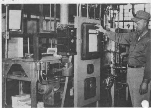
**Firing.** Firing was the most critical operation of core production. The firing temperature was approximately
