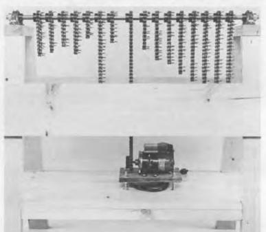
The Bicycle Chain Sieve, built in 1926 but later destroyed, is being replicated at the Computer Museum by Roberto Canepa, Andrew Kristoffy and Richard Rubinstein. This photograph shows the Museum's working model before the installation of micro-switches and a counter. The original 19-chain machine could perform 3000 tests per minute. It was used to factor the number:
