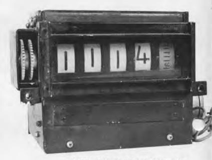
BIZMAC Clock. The BIZMAC was the result of an early attempt by RCA to produce a large-scale general-purpose computer for business applications. With its 29,000 tubes and 63,000 diodes, it was certainly one of the largest first generation computers ever built. The BIZMAC was one of the first commercial computers to use magnetic core memory. Later computers with full-scale core memories made BIZMAC obsolete.
