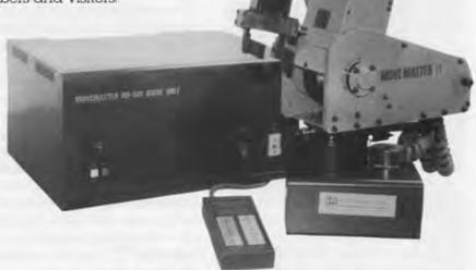
The Mitsubishi Movemaster uses its five joints and a gripper to pick up letter blocks and arrange them to spell a word typed in by the visitor. The arm is normally used for assembly or for handling chemicals.
