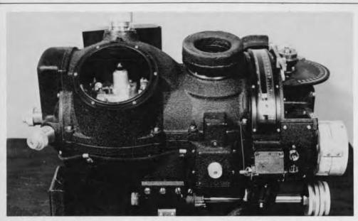
The Norden Bombsight became famous during World War II for making bombing uncannily precise—it could place a bomb inside a 100-foot circle from four miles up. Bombardiers said that it could put a bomb in a pickle barrel from 20,000 feet. When asked to verify this information,
