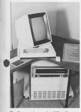
The Alto was designed in 1973 by Xerox Palo Alto Research Center as an experiment in personal computing with the goal of providing sufficient computing power, local storage, and input-output capability to satisfy the computational needs of a single user. The Alto significantly changed the office computing environment through its interactive nature and communication applications, such as electronic mail. On loan from Xerox PARC.
