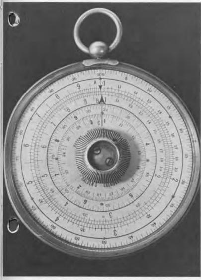
Manufactured by J. Halden and Company, London, during the 1920's, the pocket watch style calculator and slide rule has two logarithmic scales, A and B, on one side for multiplication, division and proportion which correspond to the A and B scales of an ordinary slide rule. Around the outer edge is a scale of logarithms read by a cursor. The inner circles contain a scale of square roots. The other side of the Calculex contains A and B scales for inverse proportions. Gift of Thomas McIntyre.
