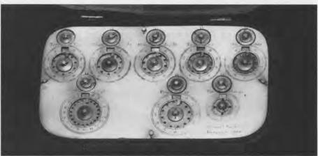
Digital Adders. Most mechanical adders use gears to "count." As you enter a number the machine "counts" the number of gear teeth that you advance. Calculating by counting is called digital calculation. The idea of using a stylus to advance gears to perform addition dates to 1642, when the French mathematician Blaise Pascal (1623-1662) invented a calculator called the Pascaline. Many mechanical calculators built for the pocket operated on similar principles.
