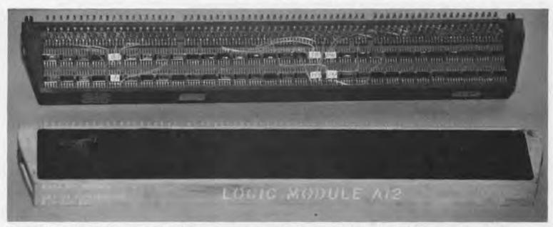
The module in the background is exactly the same as one in the foreground, but it has only been used on Earth. The Museum's prototype computer ran at Draper Labs and was used to test the routines for the in-flight machines. In space all of the components had to be totally "potted" to insure that all the parts would stay firmly in place and remain uncontaminated during space flight.
