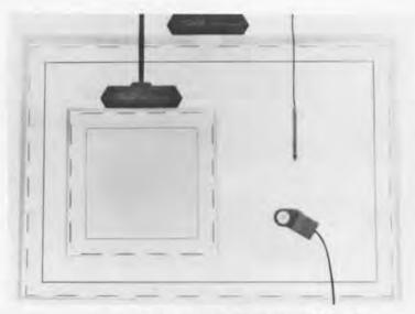
Transparent Digitizing Tablet, by Scriptel Corporation, 1984. A transparent tablet allows original artwork or photographs to be placed underneath the tablet—protected from scratching or staining. The tablet can be mounted onto a flat display screen enabling video images to be digitized. With a frosted glass finish, a slide could be back-projected onto the tablet for digitizing. A major application is the digitization of medical images, particularly X-rays.
