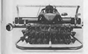
The "Blick" was the first typewriter intended to be readily portable. Designed and patented by George Blickensderfer in 1890, it was first sold in 1893. Each key had three positions, upper and lower case and a figure that positioned three levels of the printing wheel. Gift of Clark Prestia.
