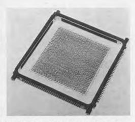
Finished Product. The final operation in the construction of a plane was the insertion of the inhibit winding and sensing wire which linked all the cores in the plane.
