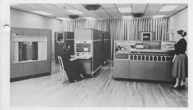
IBM 650. The IBM 650 was the most widely used first-generation computer. Hundreds were delivered between 1955 and 1959. Although the 650 as faster than other magnetic drum imputers, its high success rate was a result of a well-integrated, punched-card input and output and its adaptability to existing punched-card systems.
