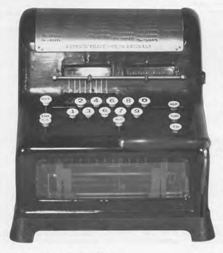
Prototype Von Reppert Calculating Machine. This artifact is truly one of a kind. It is a prototype of a calculating machine built by its inventor Richard von Reppert. Patented in 1918, the von Reppert calculator could perform "the four fundamental calculations, addition, subtraction, multiplication, and division, as well as other useful commercial work, in a practical manner." Von Reppert sold this and several other patents relating to mechanical office machines to the Underwood Company in 1920.
