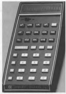
The Hewlett-Packard HP-35 was the first scientific pocket calculator. It could very quickly and accurately perform many of the slide rule functions that were too complicated for simple fourfunction calculators. It was nicknamed the "electronic slide rule." Thanks to the speed of electronic circuits, the HP-35 could calculate the logarithm of a number at the push of a button. When introduced on February 1, 1972, the HP-35 cost \$395.
