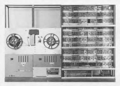
Constructed in 1966 as an unsponsored educational project of the Departments of Mathematics and Electrical Engineering at the University of California, Berkeley, the Delay Line Number Sieve performed I million tests per second. Navy surplus delay lines store the acceptable remainders for each modulus and circulate them synchronously. The machine has an idle mode in which all of the delay lines are connected in series and the data recirculated, so that the machine may be "stopped" and loaded.
