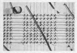
Figure 10. Detail of an early RCA memory. Note the use of decimal numbers, chosen because of the craze for decimal machines prelevant at the time.
