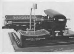
The Mignon typewriter is an indicatortype of machine, employing a stylus and a printed character table to manipulate the machine. Manufactured in Germany in 1908, the Mignon's advantage was its interchangeable letter table and type wheel, allowing typing in different languages. The Mignon is one of a gift of twenty-two typewriters from Clark Prestia. The donation represents an important part of the history of transducer equipment.
