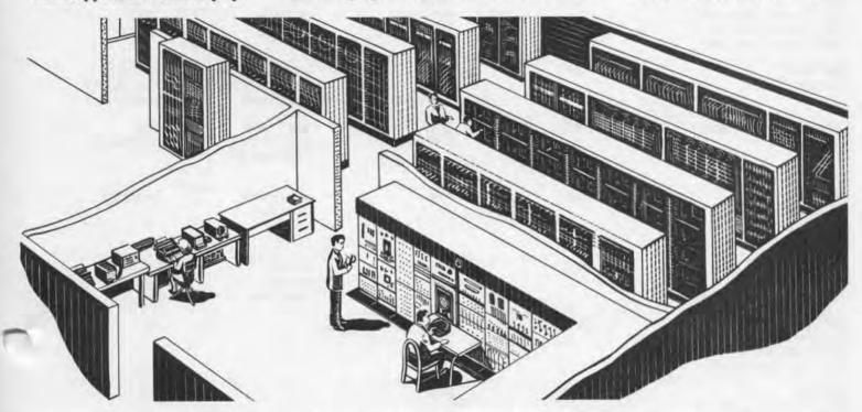
proved construction of a digital computer in 1946. A general-purpose computer could take care of not only flight simulation calculations, but a variety of other scientific and engineering applications. Whirlwind was completed in stages; the entire central machine was working in 1951.
