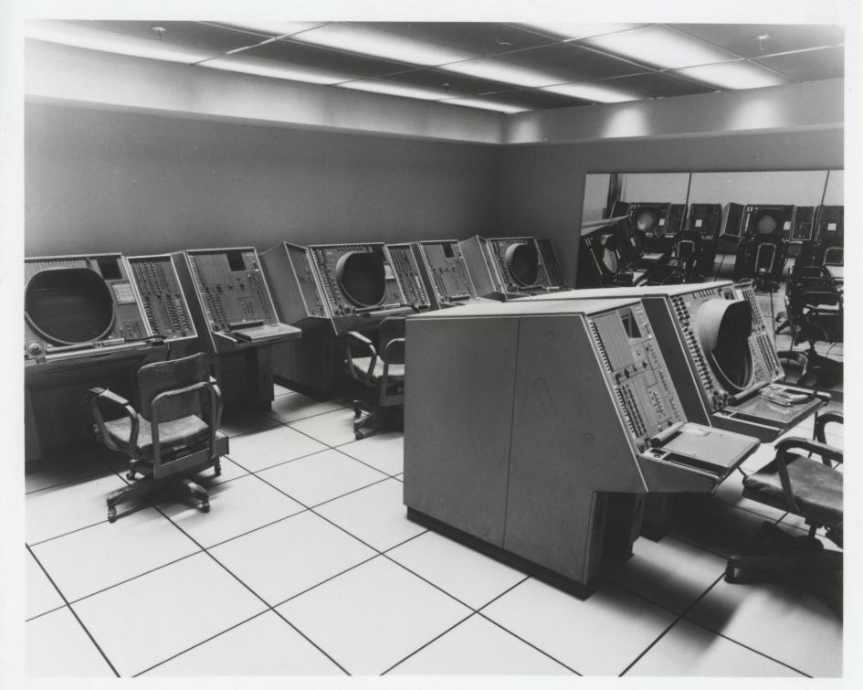
Pictured is "the Blue Room," the control room for the SAGE, the U.S. air defense system from 1958-1983. Here, Computer Museum visitors will see the oversized video display terminals that served as the first computer graphics output devices.
