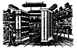
1945 ENIAC, the first all-electronic machine, was built. It was more like a calculator than a present-day computer, though, as it could not store data or programs. ENIAC stands for Electronic Numerical Integrator and Calculator.
