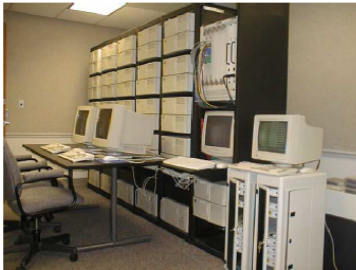
Figure 4-6. Typical Beowulf cluster configuration.
