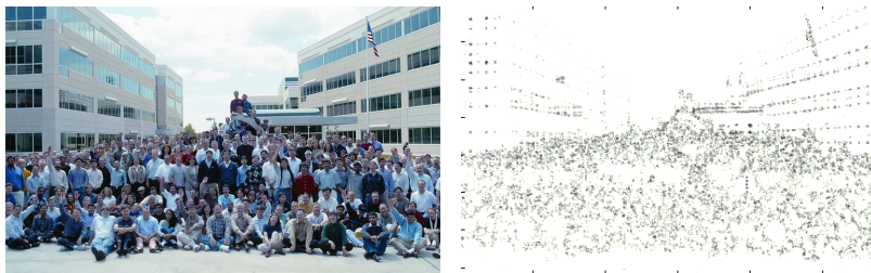
Fig. 1. An image and the result of image analysis. The darker regions are estimated to be more likely to be used as symbols in a click password. Cardinality of the password alphabet for this high-resolution image exceeds 500 symbols.
