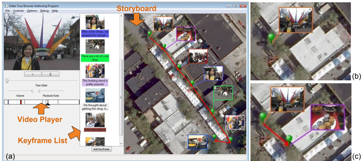
Figure 4: The authoring tool of our system. (a) The layout of the UI. (b) Adding the first keyframe to the map. (c) Adding the second keyframe to the map automatically creates a piece of tour path.
