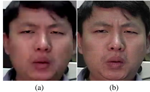
Fig. 3: Reconstructed frame 385 with (a) JVT coder (Y PSNR=32.3dB, 3144 bits); (b) the face video coder (Y PSNR=32.0dB, 2902 bits).
