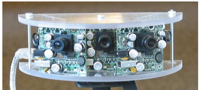
Fig. 5. The half-ring camera which consists of five 1394 fire-wire video cameras. The center camera has the smallest field of view.
