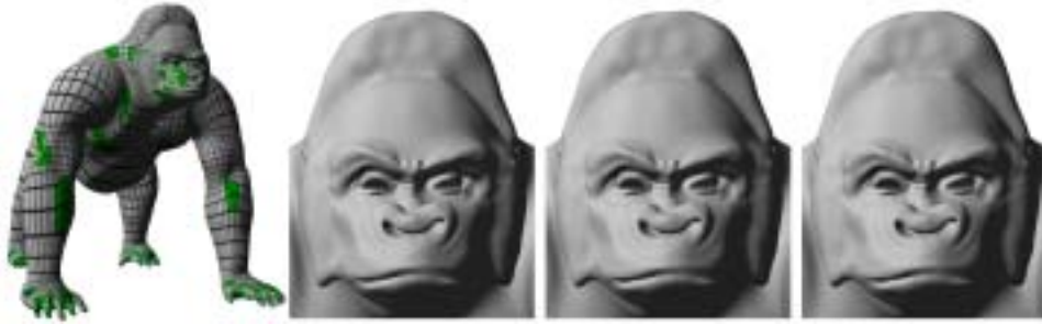
Fig. 13. A complex mesh with boundary. From left to right: Catmull-Clark patch structure, Geometry patch approximation, Geometry/Tangent patch approximation and Catmull-Clark limit surface.
