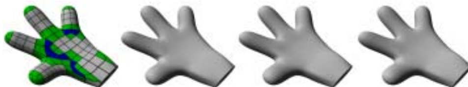
Fig. 11. An example of a mesh with a boundary. From left to right: Catmull-Clark patch structure, Geometry patch approximation, Geometry/Tangent patch approximation and Catmull-Clark limit surface using Biermann et al.’s boundary rules.
