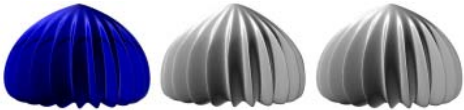
Fig. 14. A model with a valence 24 vertex at the tip composed entirely of patches with more than one extraordinary vertex (left). Our Geometry/Tangent patch approximation (center) actually appears to have a smoother profile at the valence 24 vertex than the Catmull-Clark surface (right).
