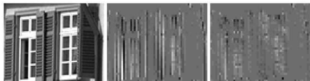
Fig. 4. Example of prediction efficiency on edges. The center image are the LH0 wavelet coefficients before prediction (amplitudes plotted as pixel intensities; zero is mid gray). The right image is after prediction.
