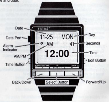
First, we need to make sure that WristMac is set to its watch-style operation and not to one of its data modes. The time button is on the left side of the watch, the bottom button. Press it several times until you see the watch display as shown.
