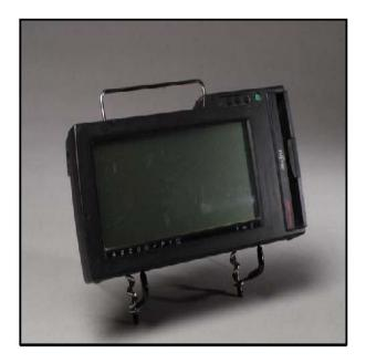
When the PoqetPad Plus was introduced in 1993, it had the same form-factor as the PoqetPad, but it had an NEC V30 processor with a speed of 16 MHz, and it used Type II PCMCIA cards. The PoqetPad Plus was destined to be the last of the Poqet products.
