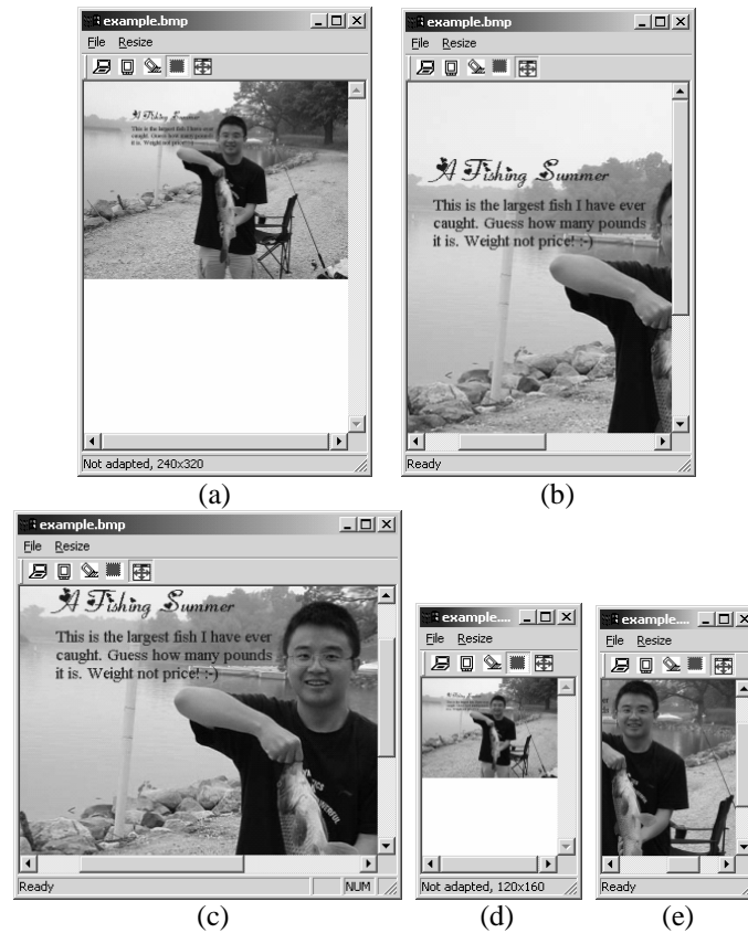
Figure 6. An example comparing the proposed attention model with the conventional approaches to adapt image. (a) direct down-sampling for Pocket PC, (b) attention-based method for Pocket PC, (c) a better adapted result by rotation for Pocket PC, (d) direct down-sampling for Smartphone, and (e) attention-based method for Smartphone
