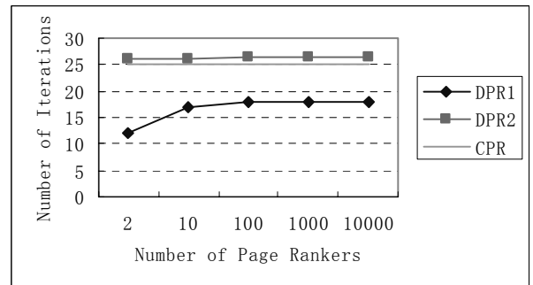
Fig.8. Comparison between different page ranking algorithms. CPR means centralized page ranking. The threshold relative error is 0.01%. ( p=1, T_1=15, T_2=15 ).
