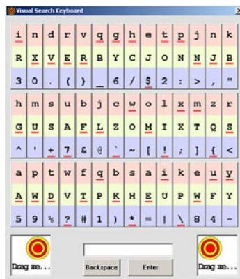
Figure 2. In the first phase of typing, the mapping phase, the user first finds the character they would like to type and notes its location. For example, if they are trying to type the capital letter “Z”, they would scan the three green rows, finding the letter on the seventh tile on the second row.
