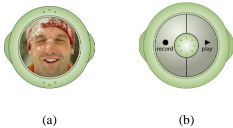
Figure 4. Magnets that allow items on fridge surfaces to be annotated: (a) indicates who created it and (b) allows voice recordings.
