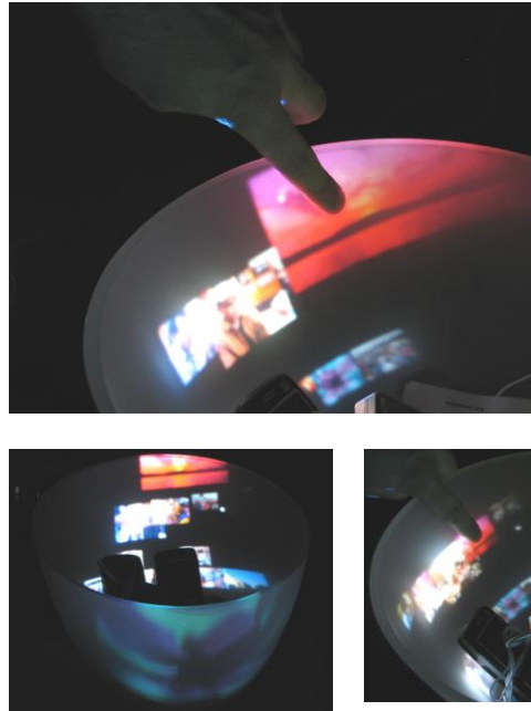
Figure 7. Current manifestation of Picture Bowl . Two data projectors project media thumbnails onto the opaque glass surface where media is visualized. We anticipate using Bluetooth and to identify individual devices and transfer content. We also intend to touch-enable the bowl, incorporating a flexible transparent capacitive overlay.
