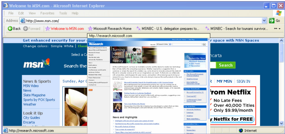
Figure 1: SmartFavourites LinkBar showing start-of-trail links (large purple stars) and page predictions (pairs of small purple stars), with the thumbnail image of the 2nd link.
