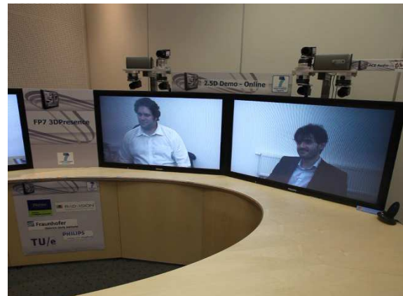
Figure 6 Correct directional eye contact and proper sense of perspective in 3DPresence project experimental setup with multi-perspective screens. Both pictures have been taken at the same time. Up: For the left conferee, gaze direction seems correct (he/she is being looked at). Down: For the conferee on the right, gaze direction perception is coherent with the left one (he/she sees the remote conferees looking at his/her left neighbor).
