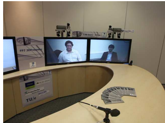
Figure 5 Exact experimental setup under development within the project for shared person and workspace telepresence using prototype multi-perspective 3D Screens, 3D capture and cloud-based interactive graphic surface.
