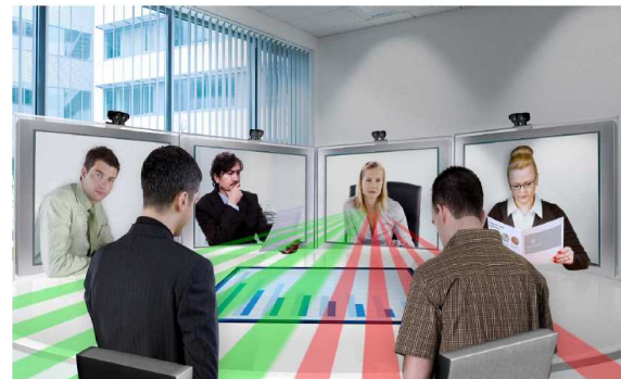
Figure 2: Evolved, more immersive, Telepresence including full 3D display system with multi-perspective experience (green and red perspective viewing cones) and integrated interactive surface for telecollaboration.
