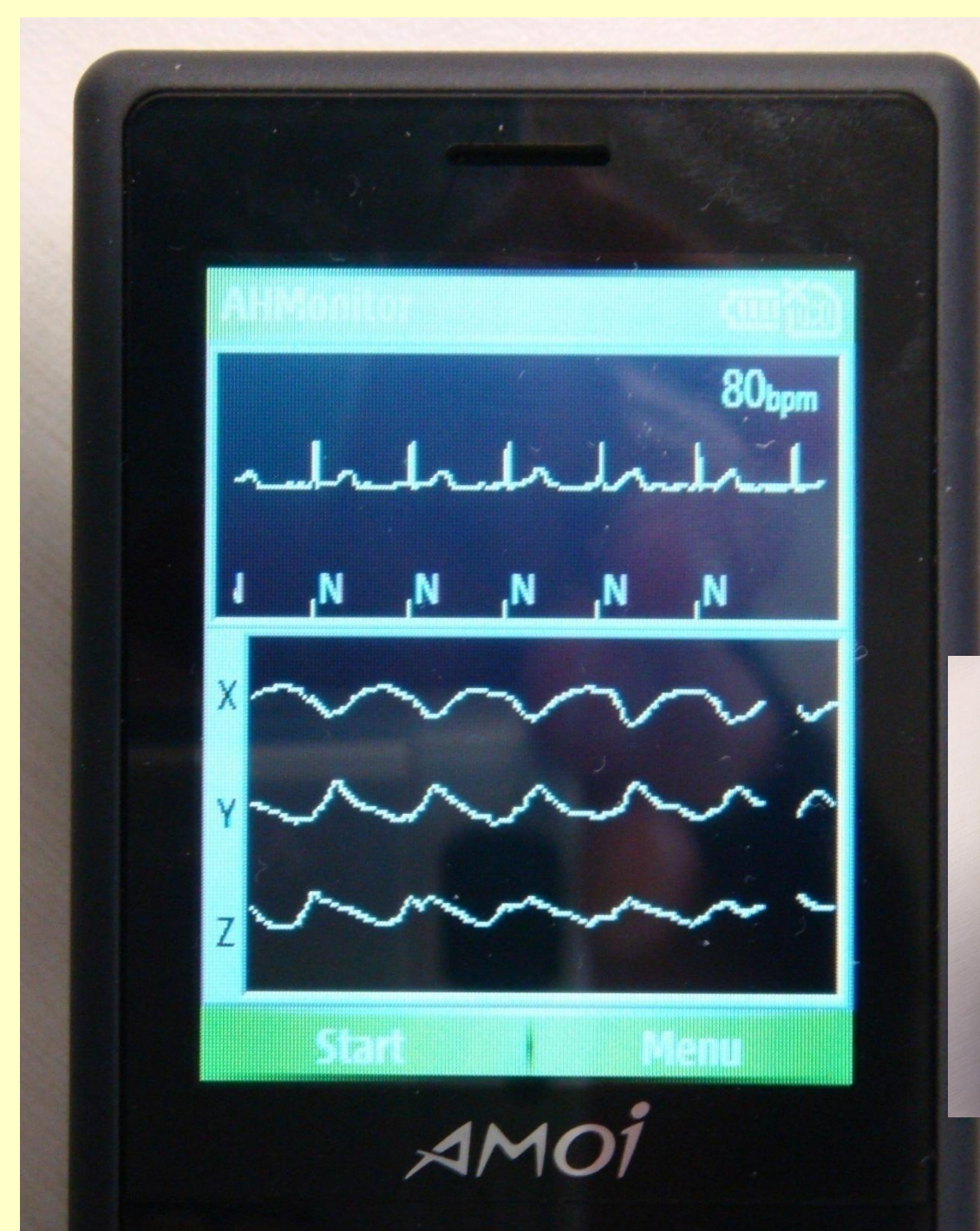
Fig. 4: The HeartToGo rule-based CVD detection user interface that includes: (top) a real-time ECG acquisition and display, plus an on-line CVD classifier; and (bottom) a 3-axis accelerometer measurement indicating the user's corresponding physical movement direction and degree of intensity.
