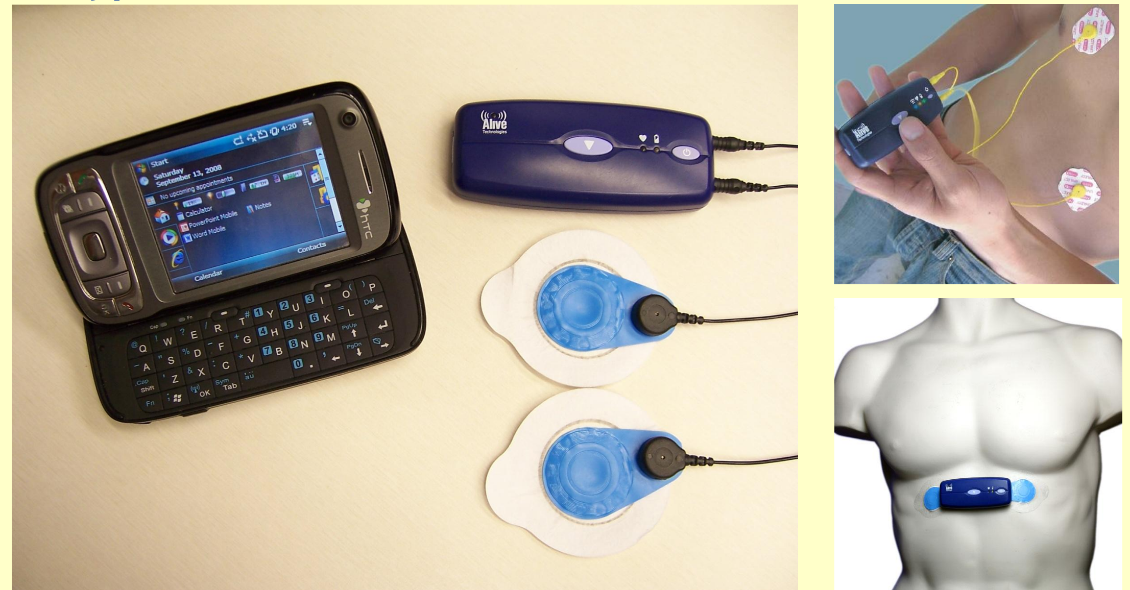
Fig. 3: The HeartToGo Platform (left), including a Microsoft Windows Mobile Smartphone with a built-in GPS and Bluetooth, plus a wearable 2-lead Alive Heart Monitor with two possible lead configurations on the chest (right).
