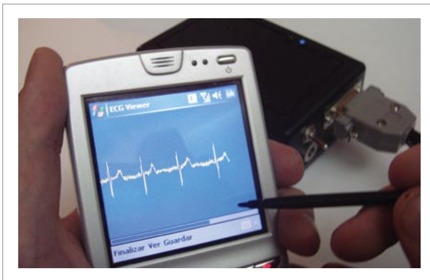
The DIKHAE system uses a smart phone that is wirelessly connected to a low-cost diagnostic tool such as an ECG module.
