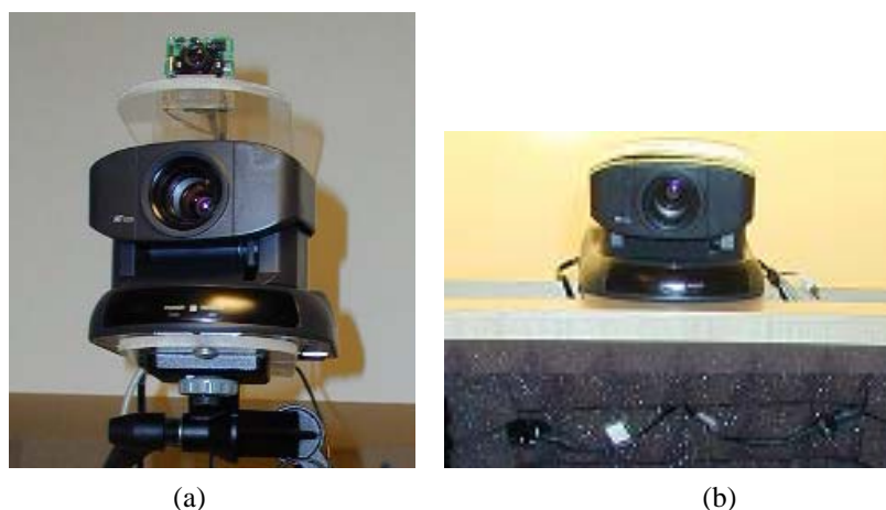
Figure 4. Devices. (a) Lecturer-tracking camera: the top portion is a static wide-angle camera; (b) Audience-tracking camera: the lower portion is a two-microphone array used to estimate sound source location
